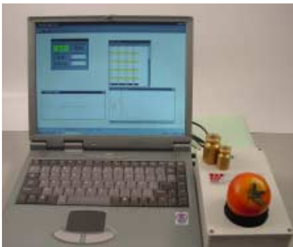
Fig. 1 Acoustic firmness sensor (AFS, Aweta, Nootdorp, The Netherlands)
